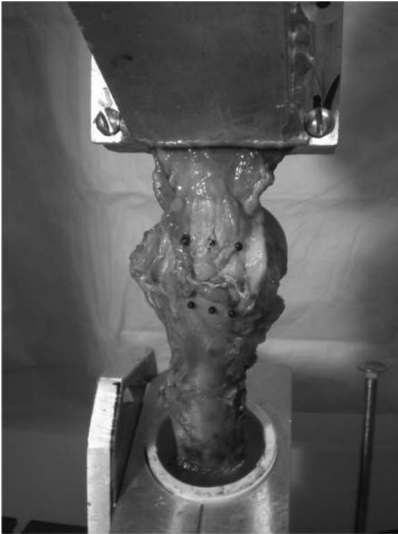
Figure 3. Mechanical testing set-up with optical markers placed.
