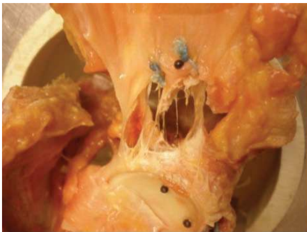
Figure 4. Glenolabral failure after pull-to-failure testing.
