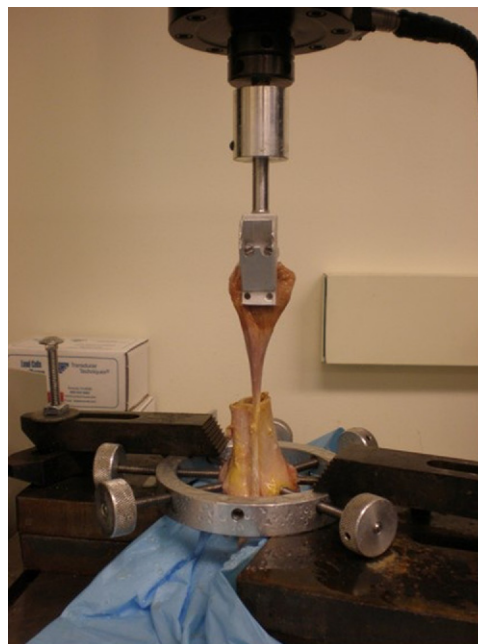
FIGURE 2. Setup of biomechanical testing of biceps tenodesis model (proximal group). The proximal humerus is inferior and the biceps tendon and muscle are superior, held by a clamp in the MTS machine. The MTS machine tested the biceps longitudinally in line with the normal pull of the biceps muscle.
